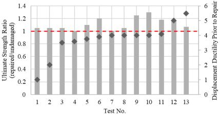
Figure 5. Post-repair ultimate strength ratio vs. maximum displacement ductility prior to repair.
