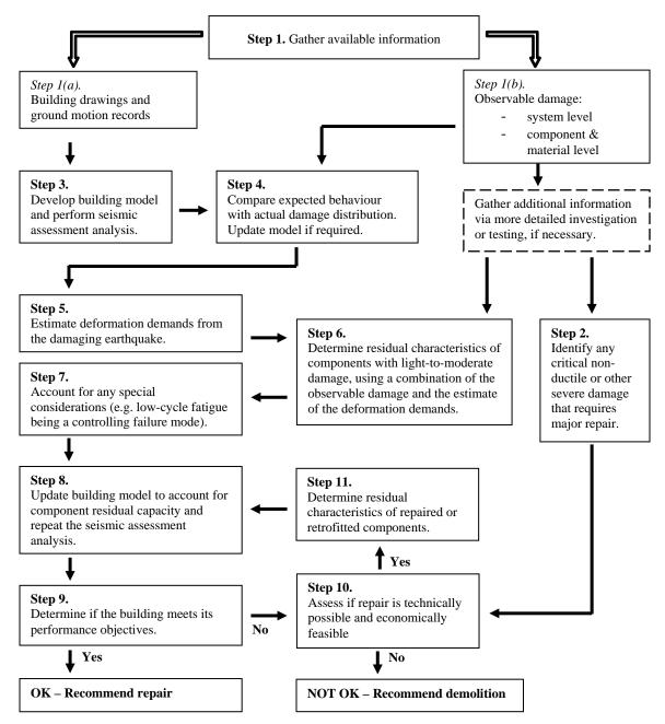
Figure 1. Proposed methodology for the detailed assessment of earthquake-damaged reinforced concrete buildings [3]
