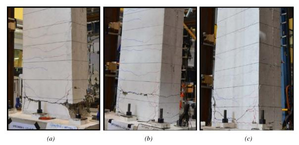
Figure 3. Pre-repair damage sate for specimen (a) LD-1-R (b) LD-2-R (c) LD-2-LER-R
